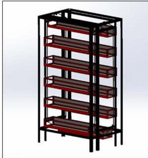
Fig.1. Vertical Carousel Storage System
